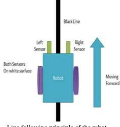
Line following principle of the robot **REFERENCE**
